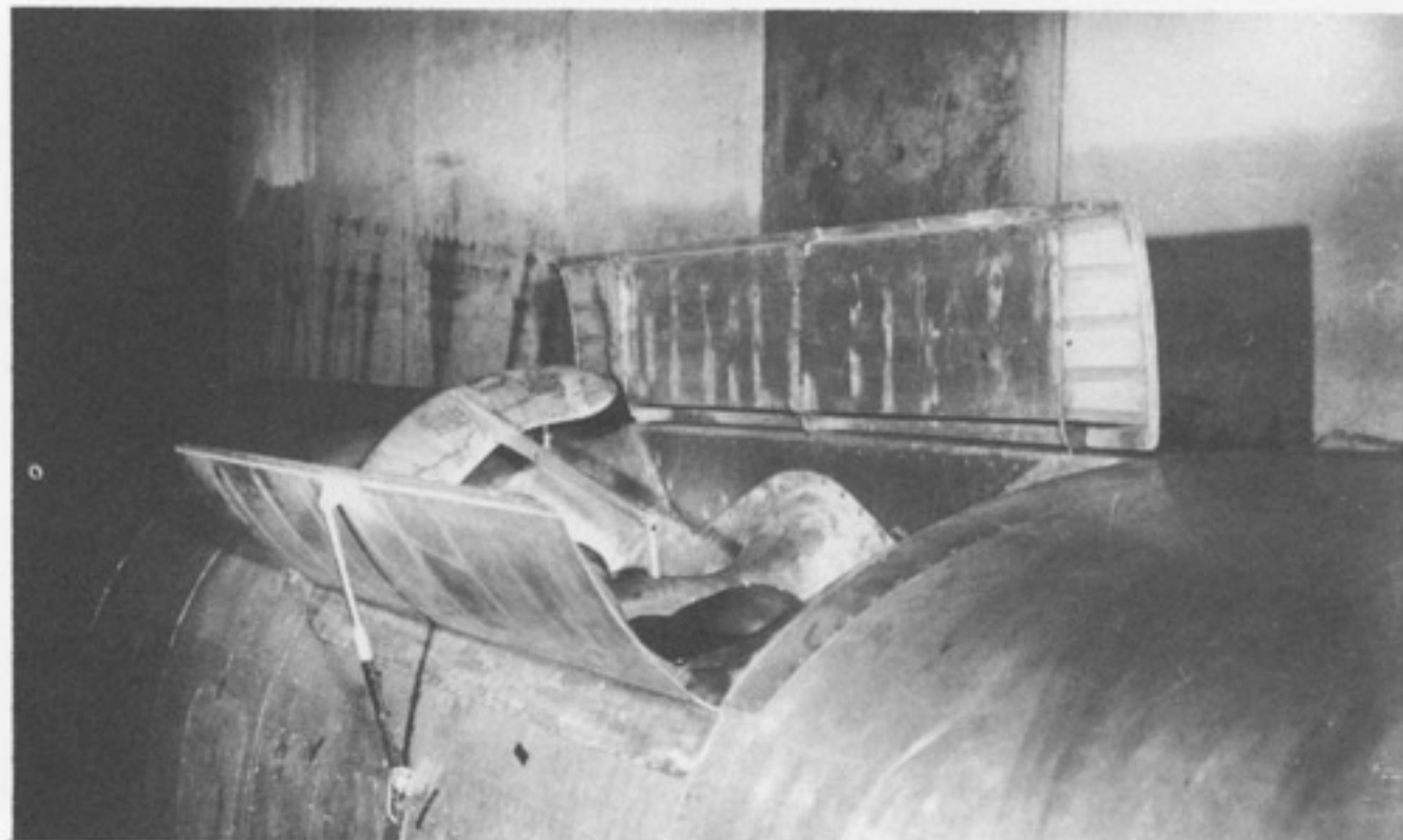
Final configuration of lift engine air intakes
