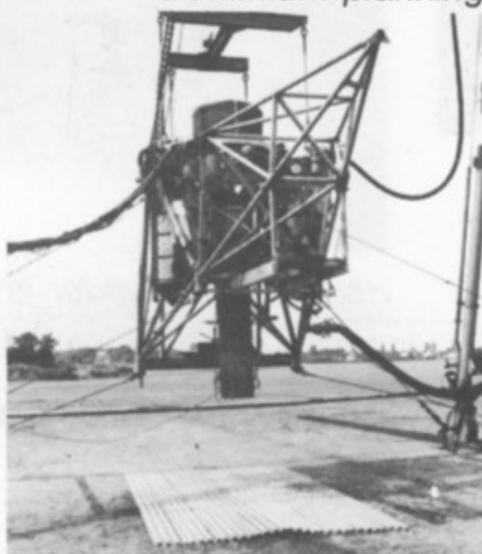
RB108 testing over aluminium planking
