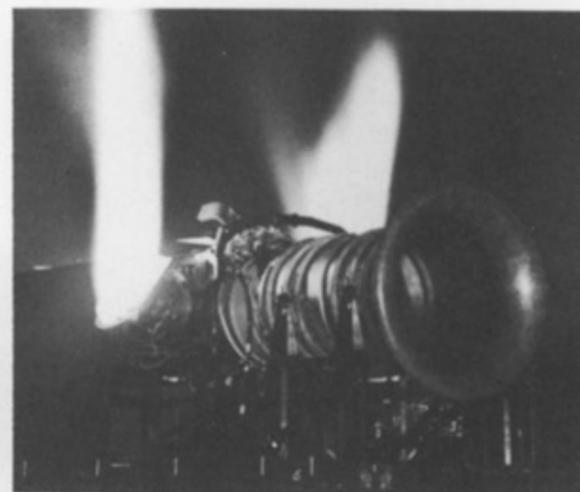
Pegasus 2 with plenum chamber burning on test
