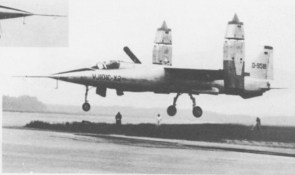
Two RB145 engines in swivelling wingtip pod
