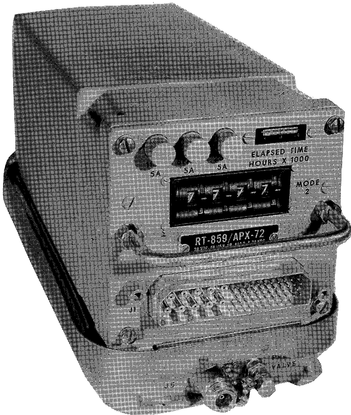
Figure 14-10. AN/APX-72 IFF Transponder
